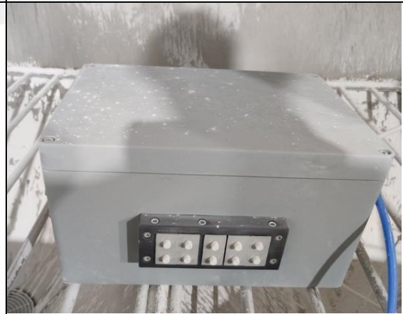
After IP5X test
