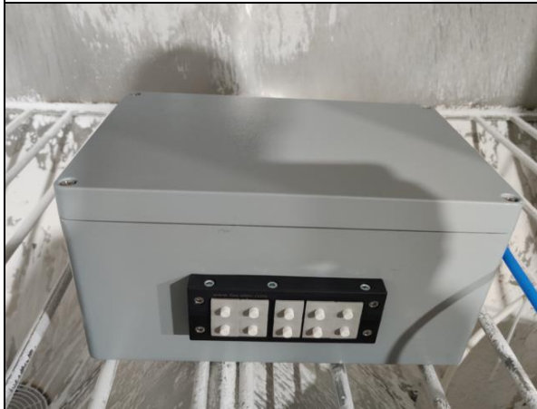
Before IP5X test
