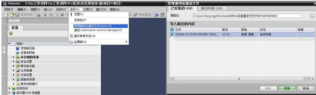
2、In PLC---Device Configuration---Network View---Hardware Catalog, select the module and drag it in, click "Unassigned", and select the PLC to be connected;
